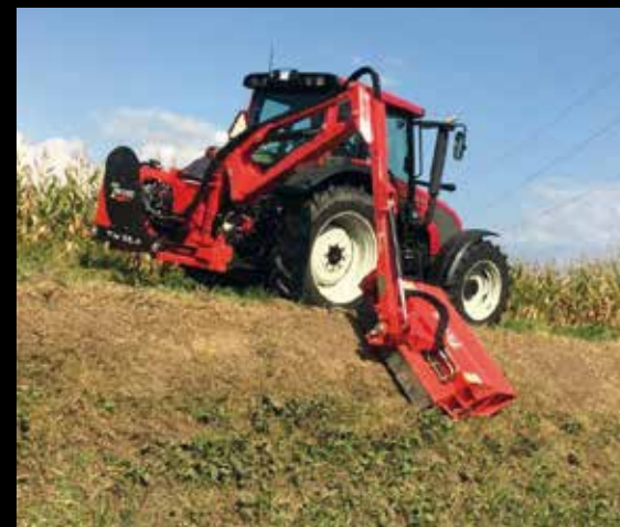
The 4-Series incorporates Hydraulic Slew. See page 21 for details
