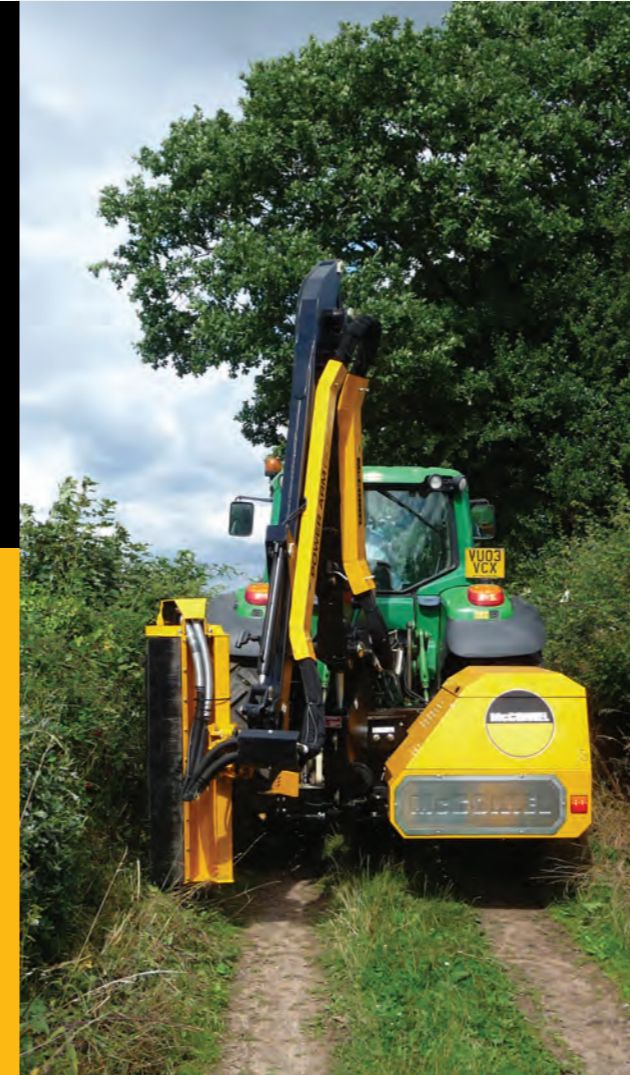
Orbitor Head Bracket enables an extra angle of movement
