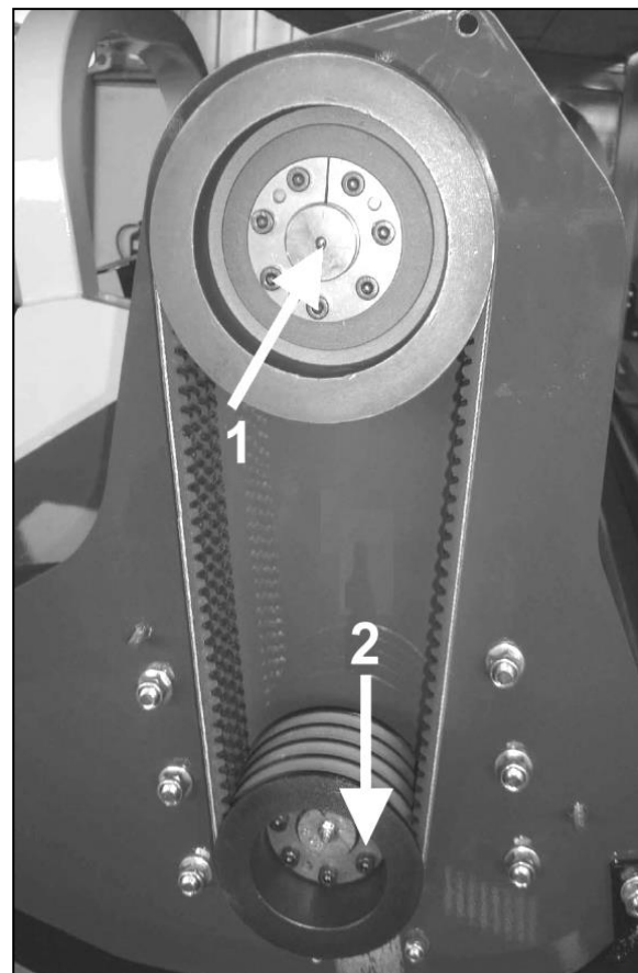
Taper Locks – check tightness on new machines after initial 2 hours of work
