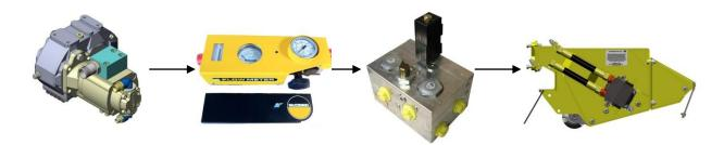
Fit the flow meter between the pump and the rotor control valve or armhead valve. Great care must be taken to ensure that the flow meter restriction control is fully OPEN initially, and is closed gradually to ensure the pressure rating of the system is not exceeded. Satisfactory pump performance will confirm the relief/control valve is at fault.
