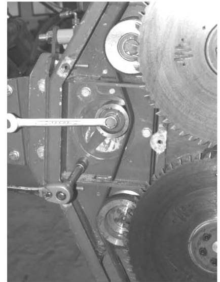
Loosen bolt and turn idler roller
