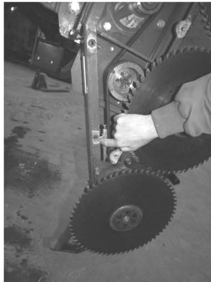
Set tension of lower belt
