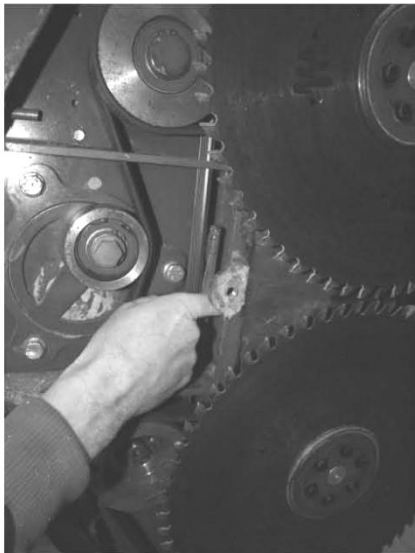
Set tension of the centre belt
