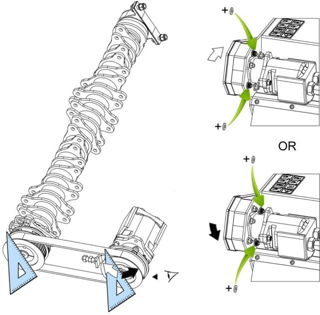
When pulleys have been correctly aligned the belt tension should be checked and if required adjusted to the correct tension; refer to belt adjustment section for details of belt tensioning procedure.
