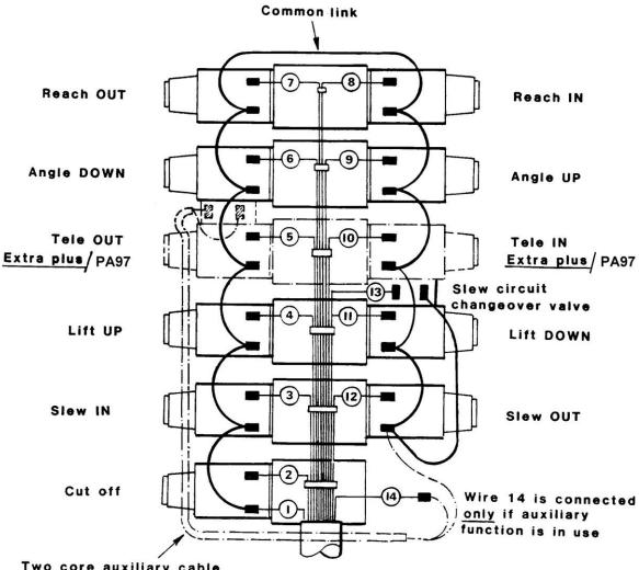
Two core auxiliary cable (if fitted).Installation of head angle float illustrated
