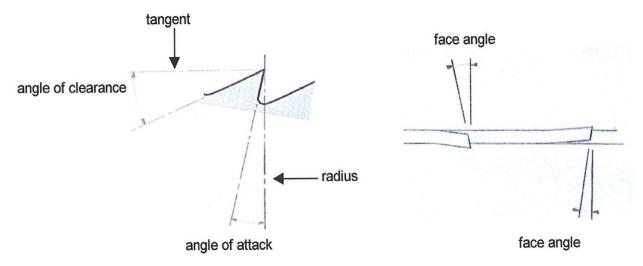
The recommended angle of attack must be set between 5° for cutting hard wood and 10° for cutting green wood.
