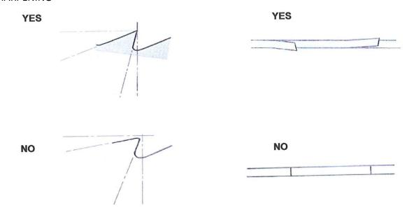
The saw teeth must be sharpened accurately to the angle of attack and the angle of clearance.
